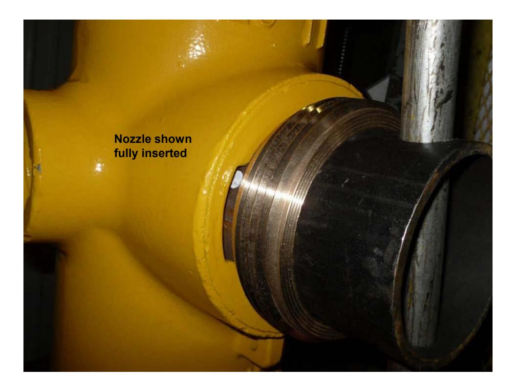
When properly installed, the nozzle set screw <u>must clear this shoulder</u> <u>before proceeding.</u>
