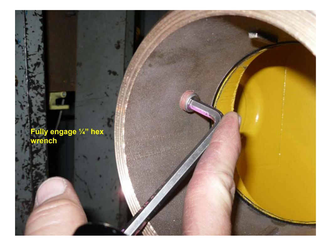
Tighten set screw (*clockwise*) until the screw is <u>between flush</u> and up to 1/8" protruding into the inside of the nozzle.
